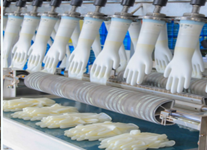
Second production line with improved technology of an auto stripping machine.
